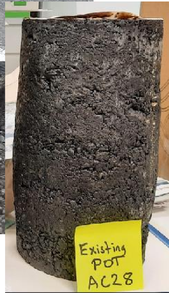
Standard AC28 RLT Mix Performance Poor and rutted (35mm)
