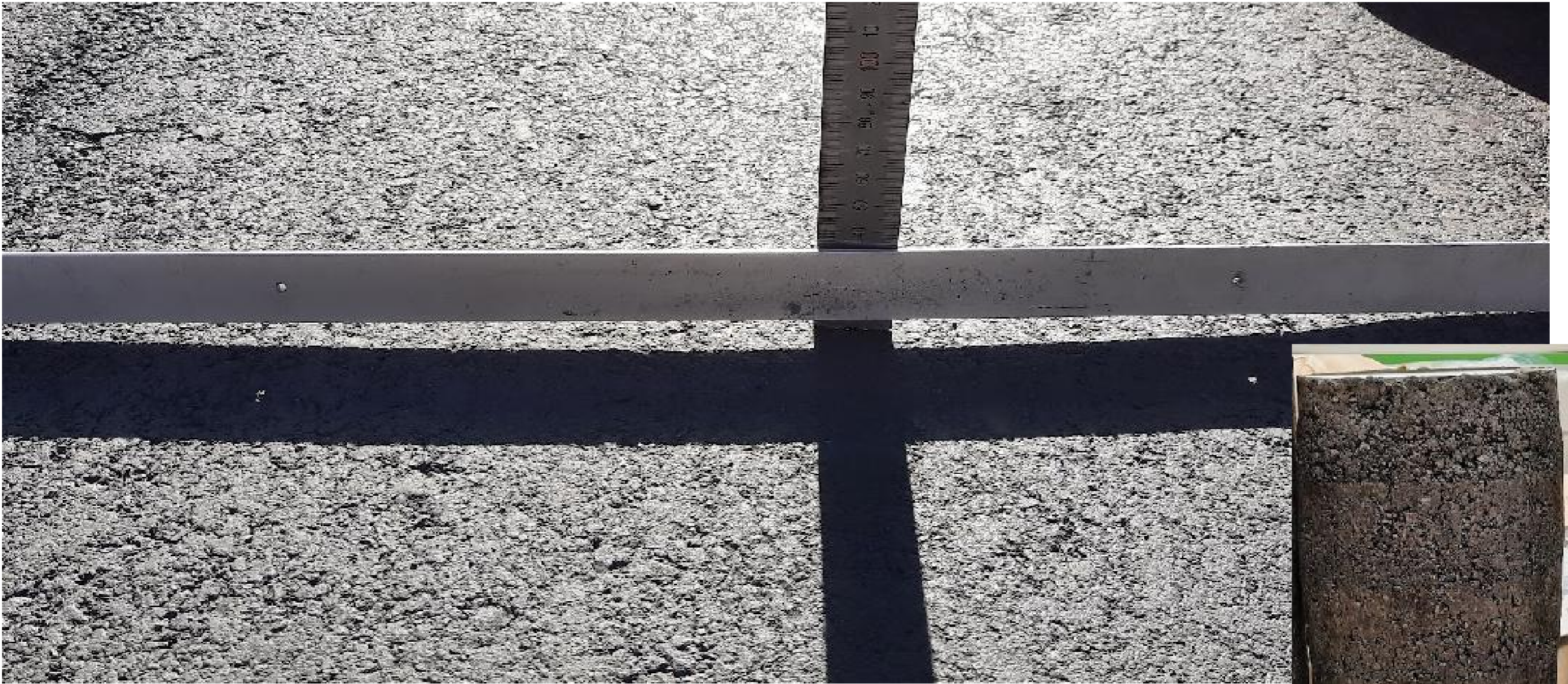
Plant Issues and RLT Mix Performance of Production Poor and rutted (15mm)
