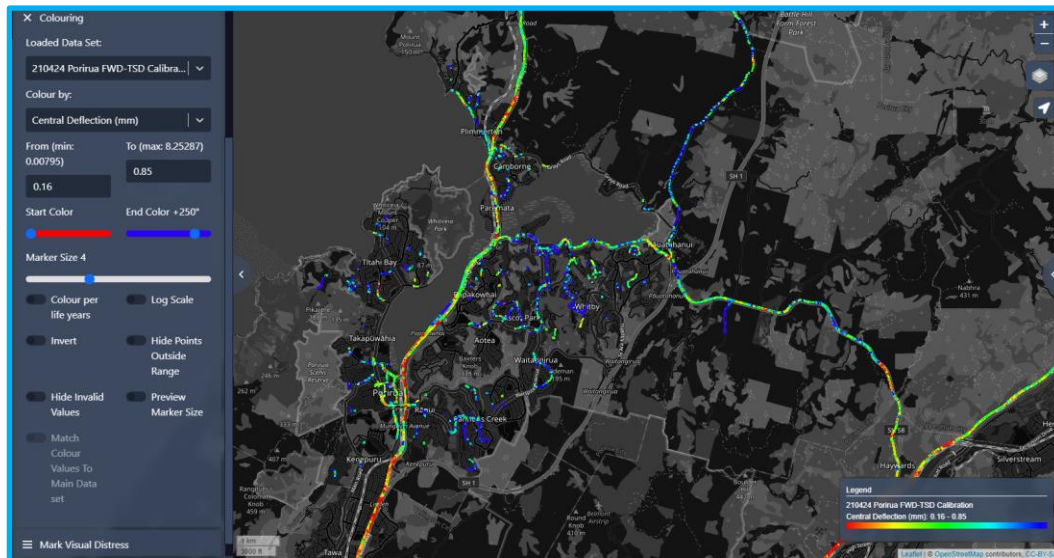
Figure 16 Reviewing FWD-TSD points coloured by Central Deflection (mm)
